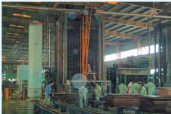
Our Team working in Chinese Plywood Factory with 40 daylight press.
